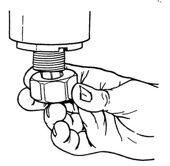
Insert Panto-collet in spindle with nut attached. Then engage nut.
