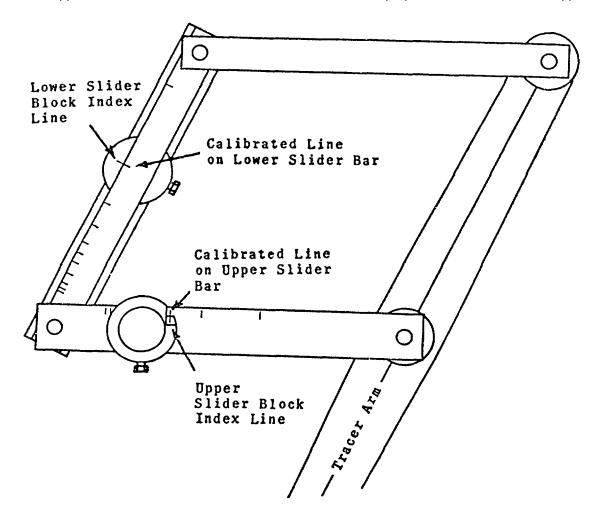
12. Refer to page 3. You will find calibrations 2, 3, 4, 5, 6 and 8 at "D". When setting the pantograph bars for any reduction, also set the slider head to the closest calibrated figure, and slide this figure into the notch on the top of cutter head mounting bracket. This will give you the maximum cutting area at the required reduction.
