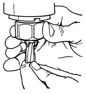
4. Insert cutter and tighten nut.
